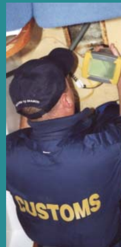
Using a "snake eye" to see into a tight spot is sometimes the only way to search a space.
