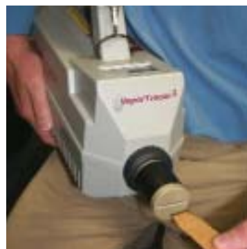
top: A swab sampler being used to pick up the possible presence of narcotic particles.
