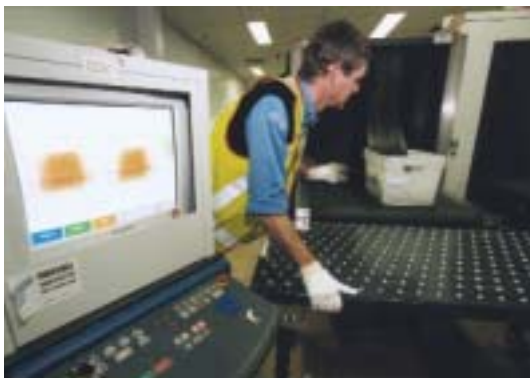
bottom: Cabinet x-ray machines used to screen postal and air cargo items - similar units are used at airports to screen passenger luggage.
